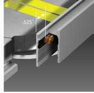
Position internal busbars to .625" from both ends of the BusRun® [refer to drawing below]
