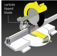
Cut BusRun® at marked location on a mitre saw with a carbide tipped blade.
