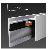
Slide the internal busbars in 1.25" from the non-cut end of the BusRun®. Busbars should be FLUSH with scrap end of BusRun.
