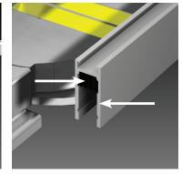
Deburr all edges and position the insulator flush with the ends of the BusRun®.
